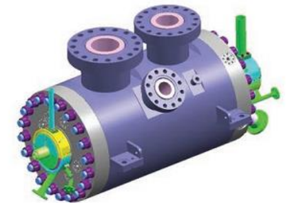
This project's team will build a prototype of the largest and highest-temperature s-CO 2 closed Brayton power cycle turbine ever constructed. The use of carbon dioxide instead of steam allows higher power-cycle efficiency and more compact cycle components. Illustration from Dresser-Rand
